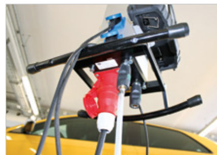
Easy handling of compressed air couplings, which are arranged at the bottom (safety compressed air couplings ISO 4414, EN 983), and the (400 V) power supply.
