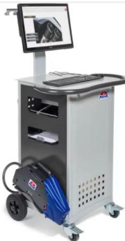
The combination tester on CONNECT trolley is designed for the measurement of petrol- and diesel-powered vehicles. In addition, low weight, compact design and short warm-up time ensure easy handling.
