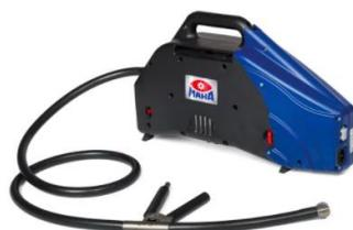
The MAHA Opacimeter is used for the measurement of diesel vehicles. The smoke opacity is tested and diagnosed in a time-saving and trouble-free manner in a partial flow procedure during free acceleration or under load of the engine. Rapid readiness for measurement and precise measurement results are the distinguishing features of the MAHA Opacimeter. Type-tested according to PTB requirements 18.09.
