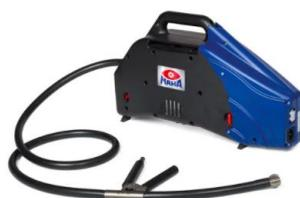
The MAHA Opacimeter on CONNECT trolley is used for the measurement of diesel vehicles. The smoke opacity is tested and diagnosed in a time-saving and trouble-free manner in a partial flow procedure during free acceleration or under load of the engine. Rapid readiness for measurement and precise measurement results are the distinguishing features of the MAHA Opacimeter. Type-tested according to PTB requirements 18.09.
