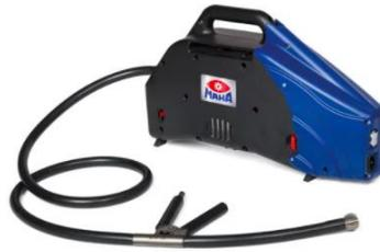
The MAHA Opacimeter on trolley is used for the measurement of diesel vehicles. The smoke opacity is tested and diagnosed in a time-saving and trouble-free manner in a partial flow procedure during free acceleration or under load of the engine. Rapid readiness for measurement and precise measurement results are the distinguishing features of the MAHA Opacimeter. Type-tested according to PTB requirements 18.09.
