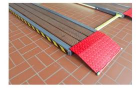
The two post inground lift, with runway, lifts cars of up to 3.5 t.
